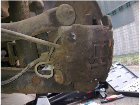
4. Hose it off with WD40. Lots of it. You can see the calliper pins now. What you need to do is remove the 2 shiny cotter pins you can see, then take a punch and a BIG hammer and whack the crap out of the pins from this direction. This can be EXCEPTIONALLY difficult.
