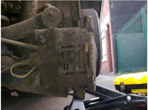
3. This is what it looks like from behind. If you want to take the calliper off, you need to remove the bolt at the bottom and the allen bolt that's behind the cap at the top (the big rubber cylinder). Notice the pins? No? That's behind a load of crud.
